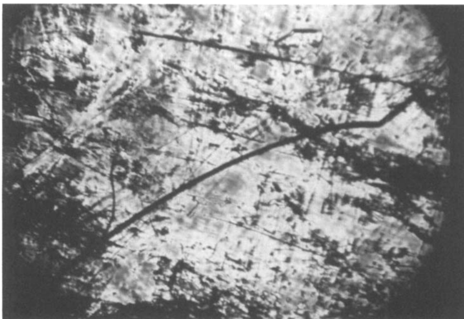
Fig. 7. 4-butoxy,4'-chloroazobenzene, T=84^{\circ}\text{C} , marble texture. See Color Plate V.
